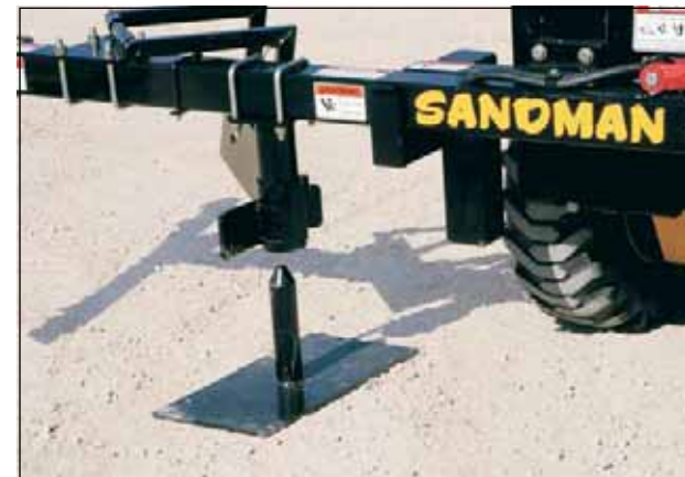
The parking stand is used when Sandman is not attached to a loader.
