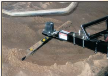
Sandman's rotary arm is driven by a heavy duty hydraulic motor. It sweeps bedding material to the front of the stall.
