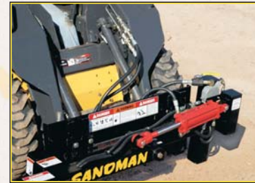
One set of hydraulic couplers run the Sandman's rotary motor and boom arm.
