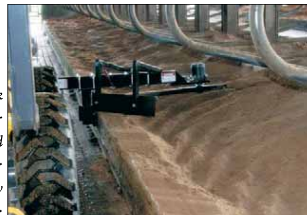
Heavy duty curb guide holds rotating arm in the center of the bedding area.
